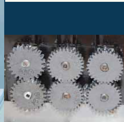
Strong, durable drive mechanism with metal gearwheels.
